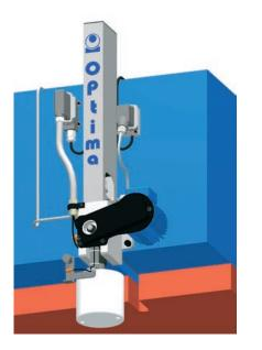
Fixing is a chieved with four hexagon heads crews with flange (DIN 6921), M10x30, strength class 8.8 and two spring dowelpins 8.8 (DIN1481) Ø8x20 (not included).
